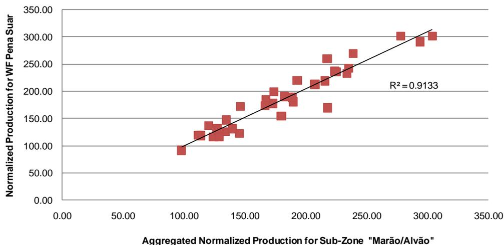
Figure 3 - Correlation between aggregated Normalized Production for Sub-Zone “Marão/Alvão” and R-WF “Pena Suar”
