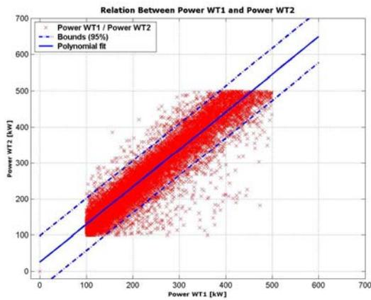
Figure 3-Filtered power correlation cross plot
