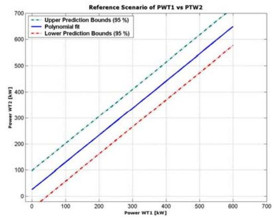
Figure 4-Pattern for the filtered power correlation
