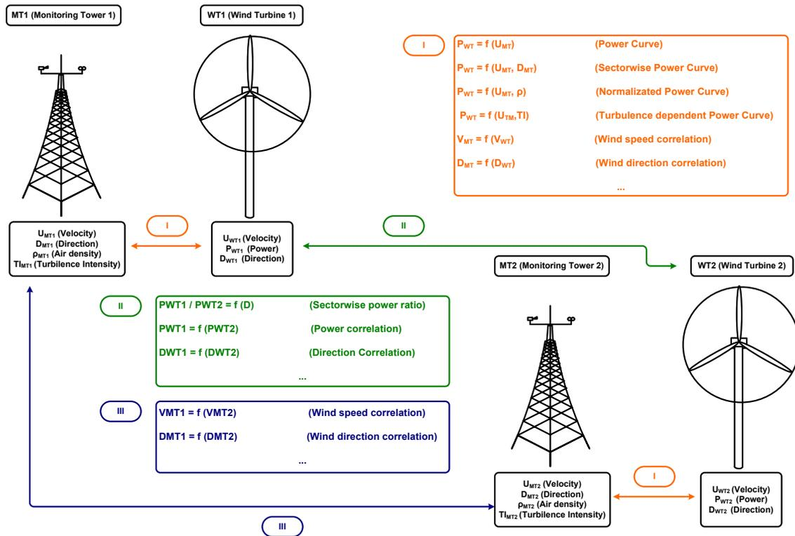
Figure 1 – Schematic representation of the proposed methodology
