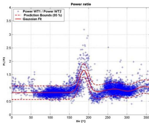
Figure 6 – Plot of filtered sectorwise power ratio
