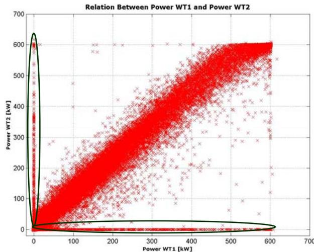
Figure 2 – Power cross correlation between two neighbouring wind turbines
