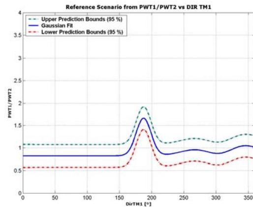
Figure 7 – Pattern for the filtered sectorwise power ratio
