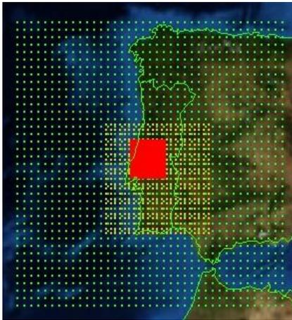
Figure 2 - Grid placement for Portugal – Simulation 2, outer grid - green, intermediate grid – yellow, inner grid - red.
