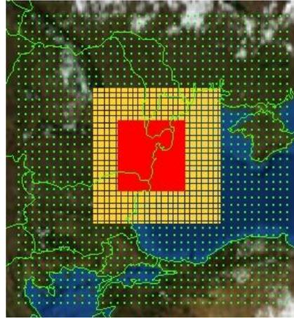
Figure 4 - Grid placement for Romania, outer grid - green, intermediate grid – yellow, inner grid - red.
