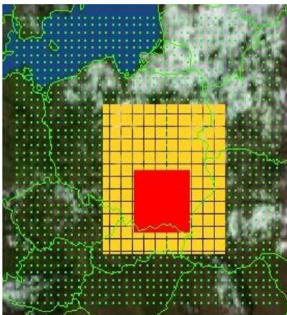
Figure 3 - Grid placement for Poland, outer grid - green, intermediate grid – yellow, inner grid - red.
