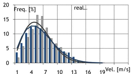
Figure 6 - Wind Speed Histogram, station (blue), WRF (grey).
