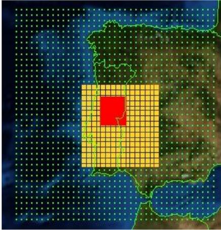
Figure 1 - Grid placement for Portugal – Simulation 1, outer grid - green, intermediate grid – yellow, inner grid - red.
